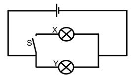
Bulb **X** has a resistance of 4  $\Omega$  and bulb **Y** has a resistance of 2  $\Omega$ .
