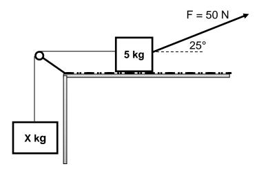
The 5 kg block accelerates at 3 m·s<sup>-2</sup> TO THE LEFT and the coefficient of kinetic friction ( $\mu_k$ ) between the 5 kg block and the surface is 0,2. Ignore the effects of the air resistance.
